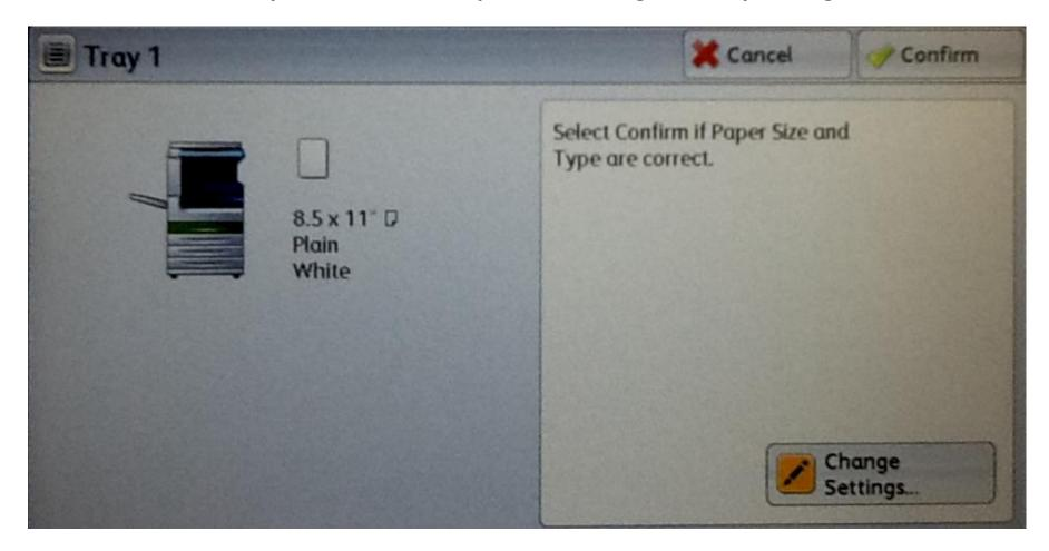
Adjust the paper size, paper type, and the color of the paper as needed by selecting Change Settings button and confirm the changes.
