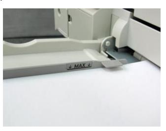
2. Place the media onto the tray. Paper must not be loaded above the max line. The paper settings for the tray are going to display on the touch screen. Confirm or change the Type of paper, the Size, and the Color of Paper in the tray.
